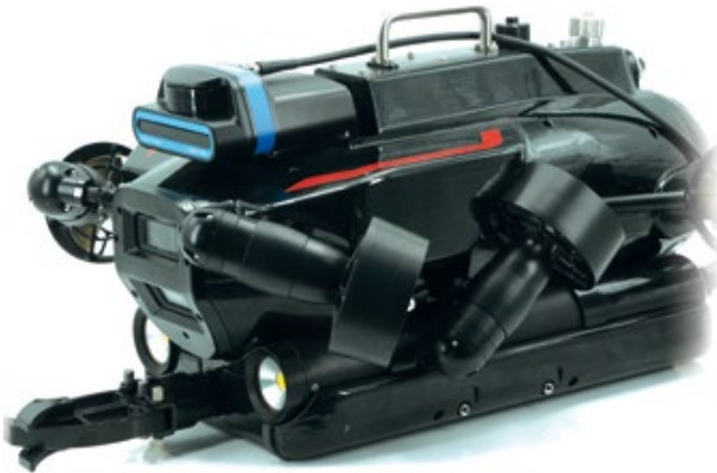
FIFISH PRO V6 equipped with the 2D Imaging Sonar & Robotic Arm (Courtesy of QYSEA)
