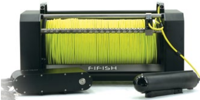
Onshore Power Supply System (OPSS) compatible with all FIFISH Underwater Robots (Courtesy of QYSEA)
